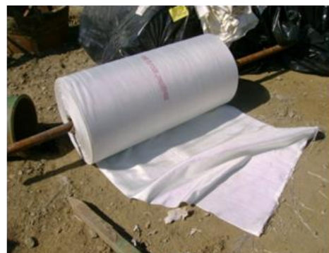
Figure 4. Typical woven seamless encasement as delivered to the site before installation.
