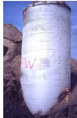
Figure 11. Typical geotextile encasement failure at a seam (Di Prisco et al. (2006)) (top photo) and stand-alone in-air seamless test GECs (bottom photos)
