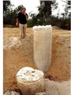
Figure 11. Typical geotextile encasement failure at a seam (Di Prisco et al. (2006)) (top photo) and stand-alone in-air seamless test GECs (bottom photos)
