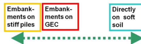
Figure 10. Position of the GEC System between two extrema: embankments on rigid elements and embankments without any support.
