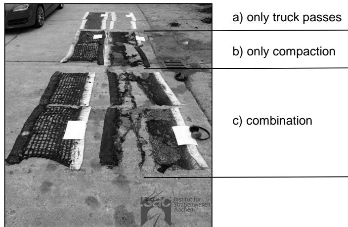
**FIGURE 2 Results of Installation Damage Test (Left Polyester Grid, Right Glass Fibre Grid) [14]**
