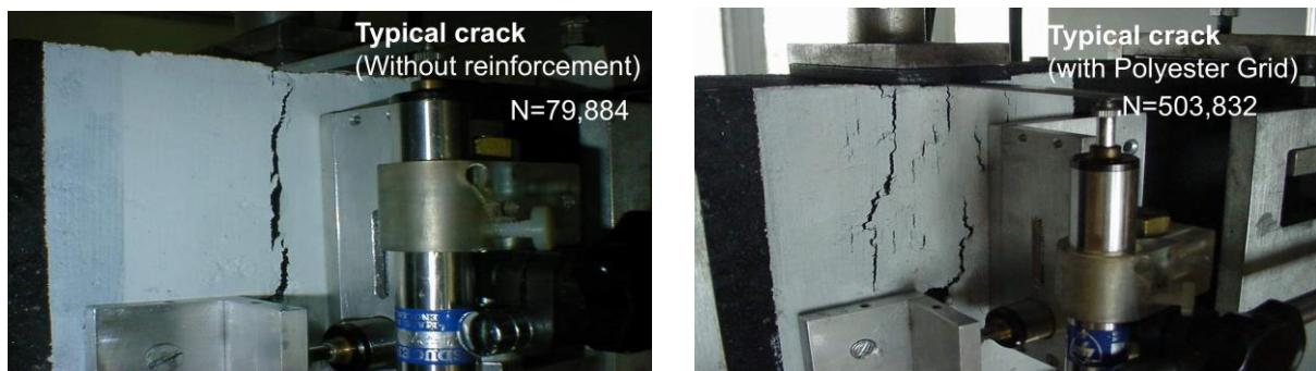
**FIGURE 3c. Comparison of Beams with and without PET grid: Typical Cracking Patterns and the Number of Cycles Conducted Before the Cracks Reached the Surface (Bending and Shear mode) [1]**
