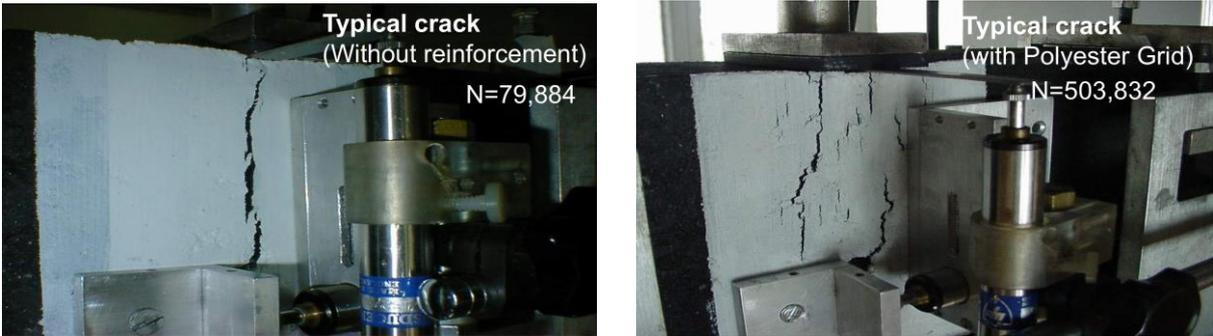
**FIGURE 3c. Comparison of Beams with and without PET grid: Typical Cracking Patterns and the Number of Cycles Conducted Before the Cracks Reached the Surface (Bending and Shear mode) [1]**
