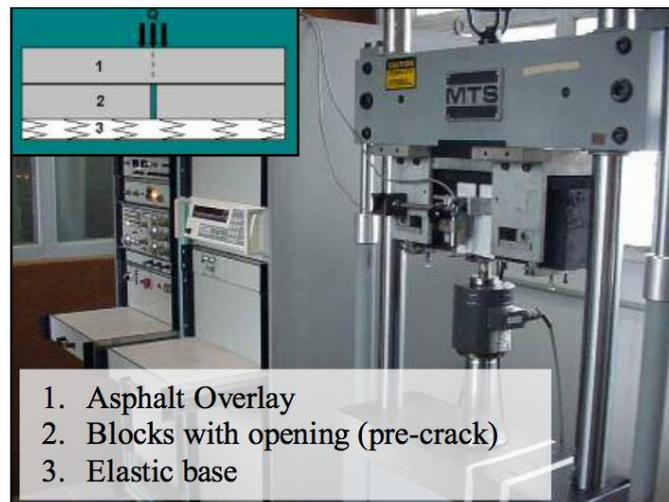
**FIGURE 3b. Test Set-up [1]**
