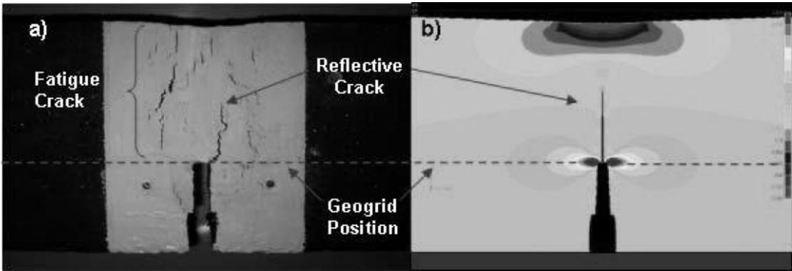
**FIGURE 4. Comparison between Laboratory and Numerical Simulation Results [1]**
