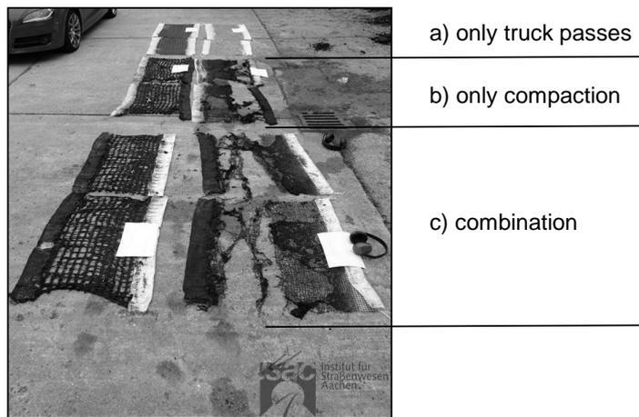
**FIGURE 2 Results of Installation Damage Test (Left Polyester Grid, Right Glass Fibre Grid) [14]**
