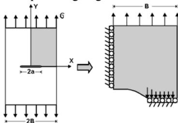
Fig.6 – Schematic Showing lines of symmetry for a middle crack tension specimen.
