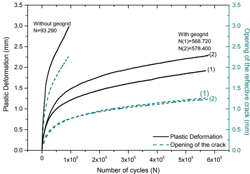
Fig.5 – Fatigue test result – Pre-crack opening 3mm (Shear).
