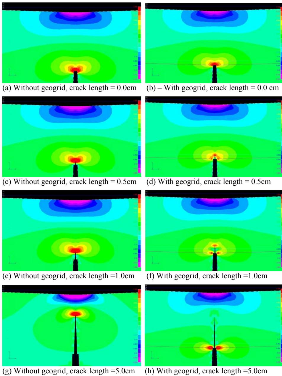
**Fig. 7-** Process zone formed by growing crack (tensile stress in the beams)
