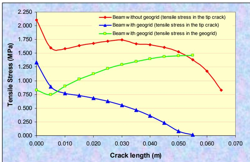
Fig. 8 – Tensile stress in the beams, with and without geogrid.
