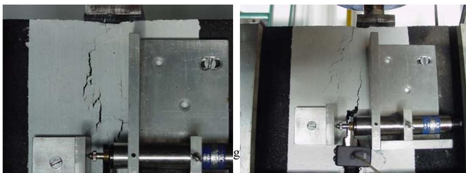
**Fig.3** - Beam with geogrid: cracking pattern in the end of test (bending and shear mode)
