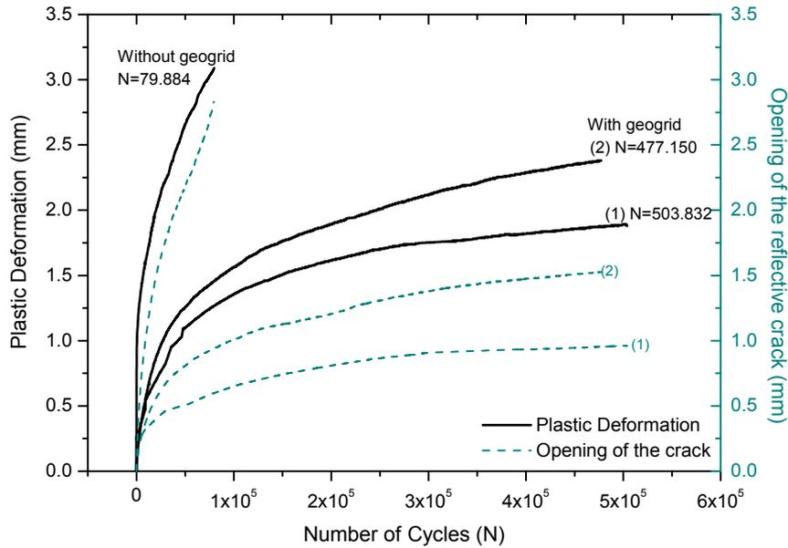
**Fig. 4** - Fatigue test result – Pre-crack opening 3mm (Bend).
