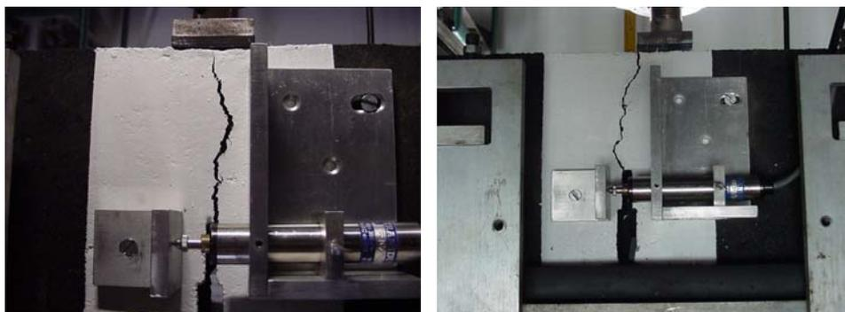
**Fig.2** – Beam without geogrid: cracking pattern in the end of test (bending and shear mode)
