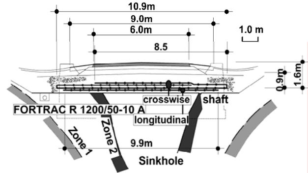
Figure 3. Schematic cross-section of the sinkhole bridging system.
