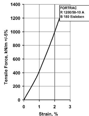
Figure 4. Tensile force/strain graph for the Fortrac® 1200/50-10 A.
