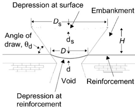
Figure 2. Analysis model in accordance with BS 8006 (BSI 1995).
