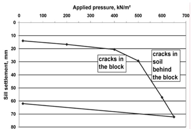
Figure 10. Settlement of the loading block in Test 2
