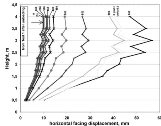
Figure 12. Displacement of the measured points on the facing for Test 2
