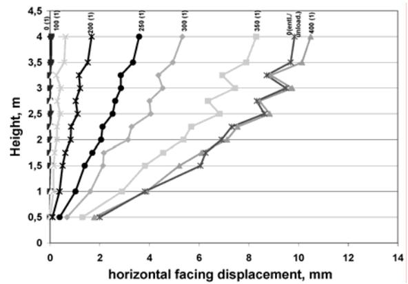
Figure 11. Displacement of the measured points on the facing for Test 1
