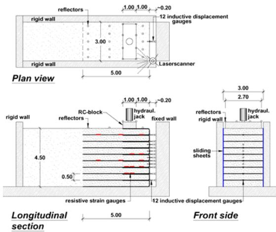
Figure 5. Schematic of the test
