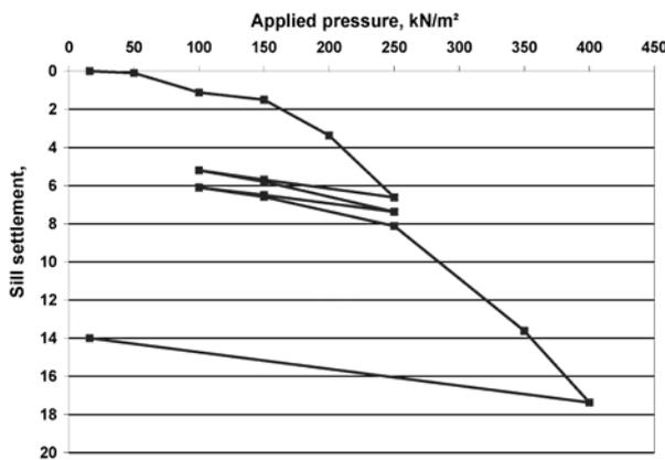
Figure 9. Settlement of the loading block in Test 1
