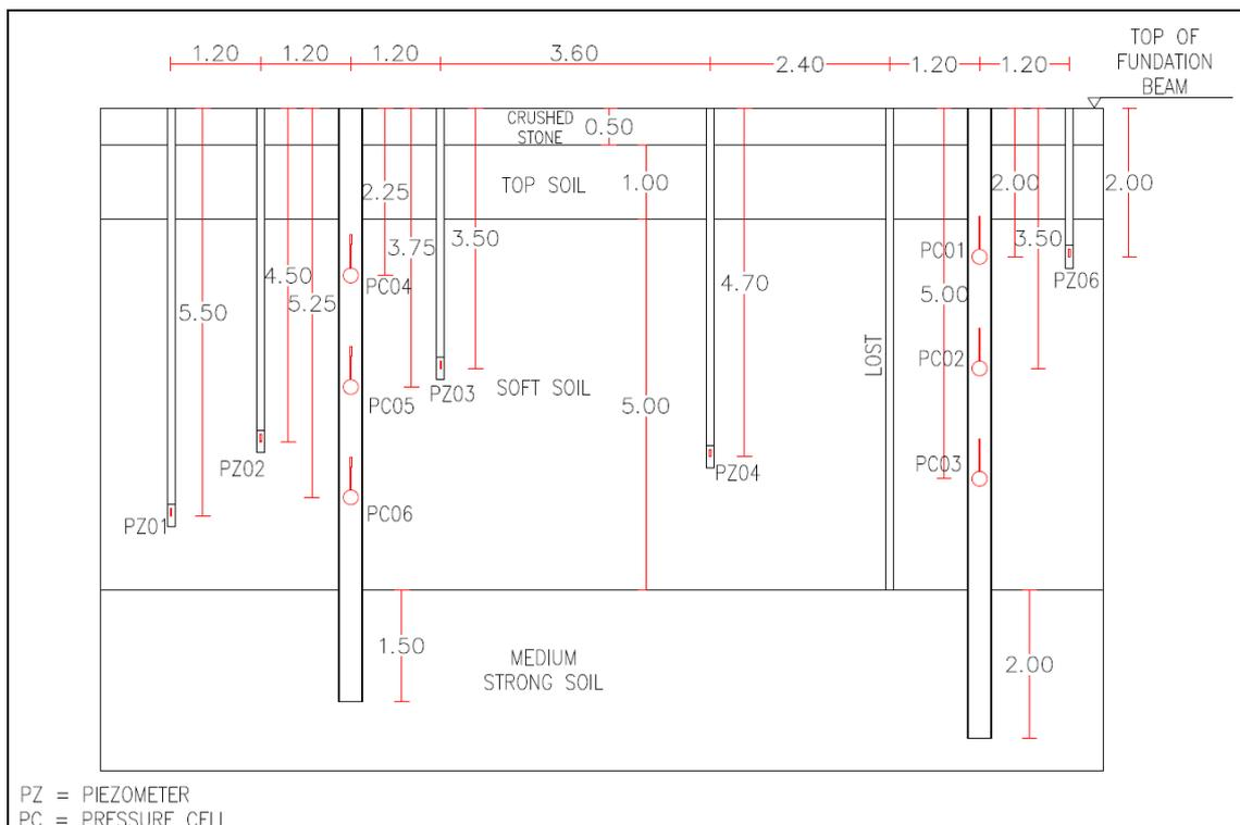
Figure 2. Instrumented cross-section.
