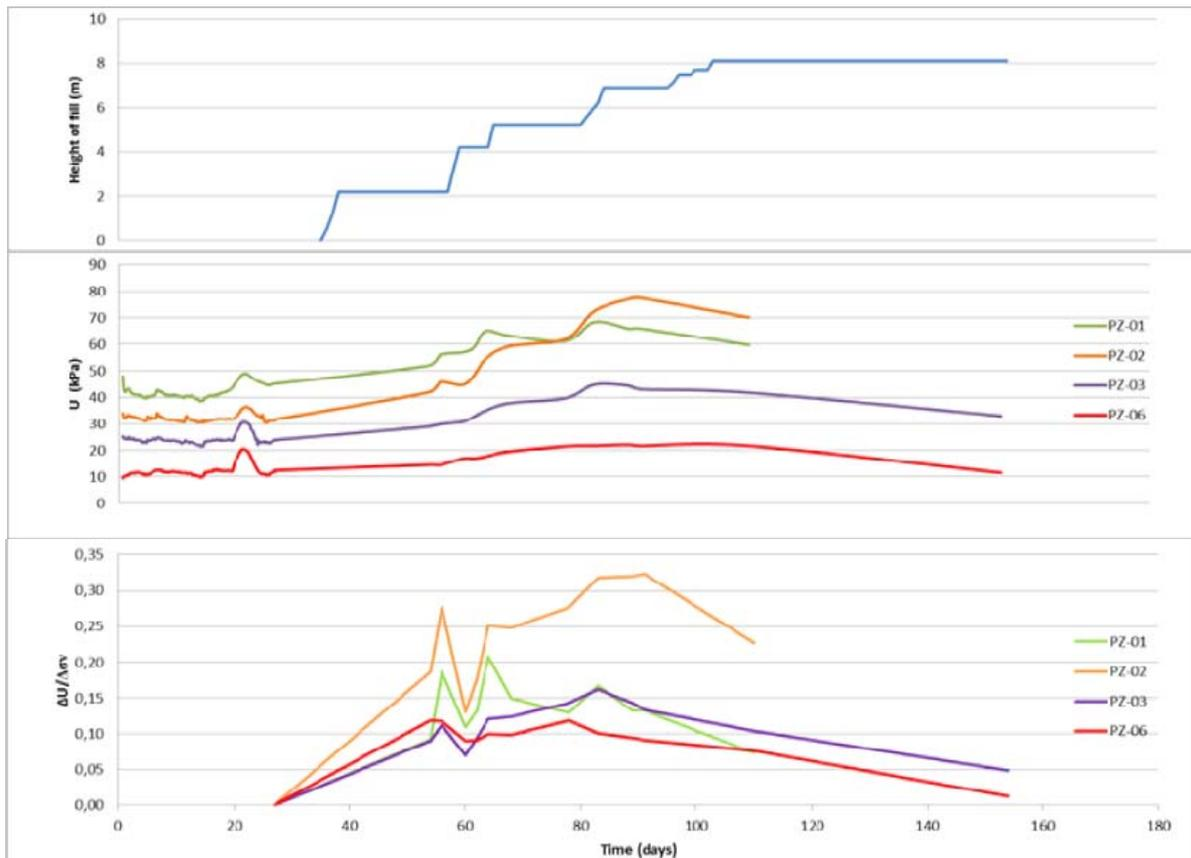
Figure 5. Variation of pore water pressure with time.
