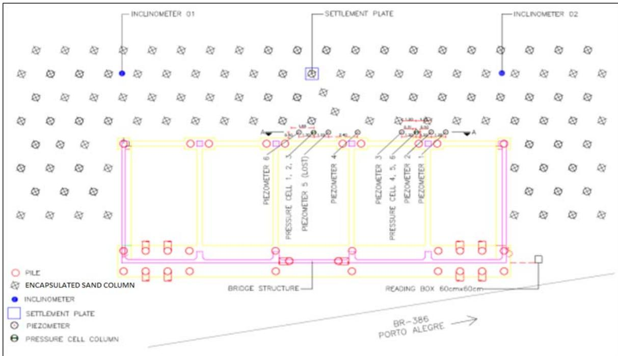
Figure 3. Plan view of the columns and instrumentation location.
