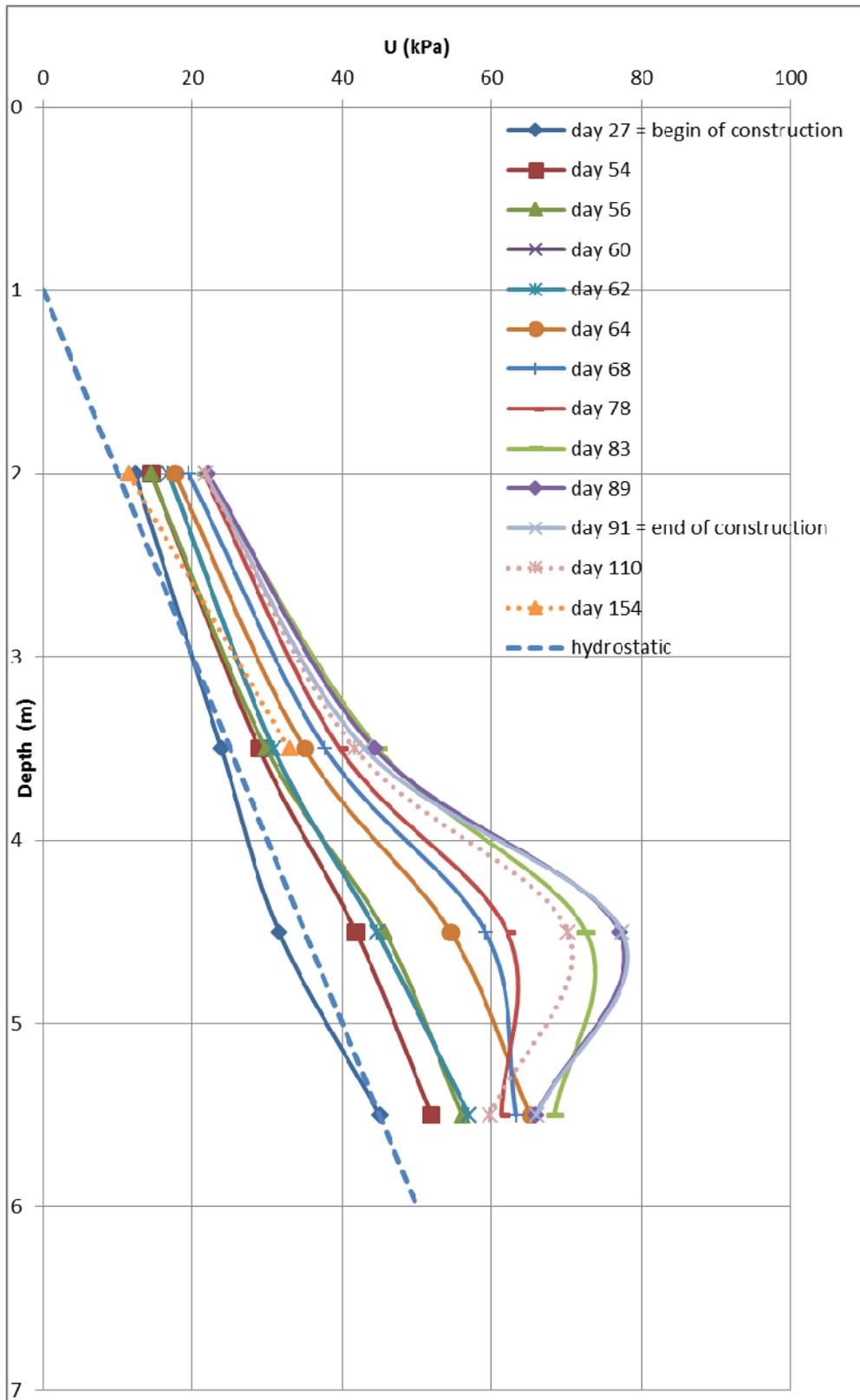
Figure 6. Variation of pore water pressures with depth.
