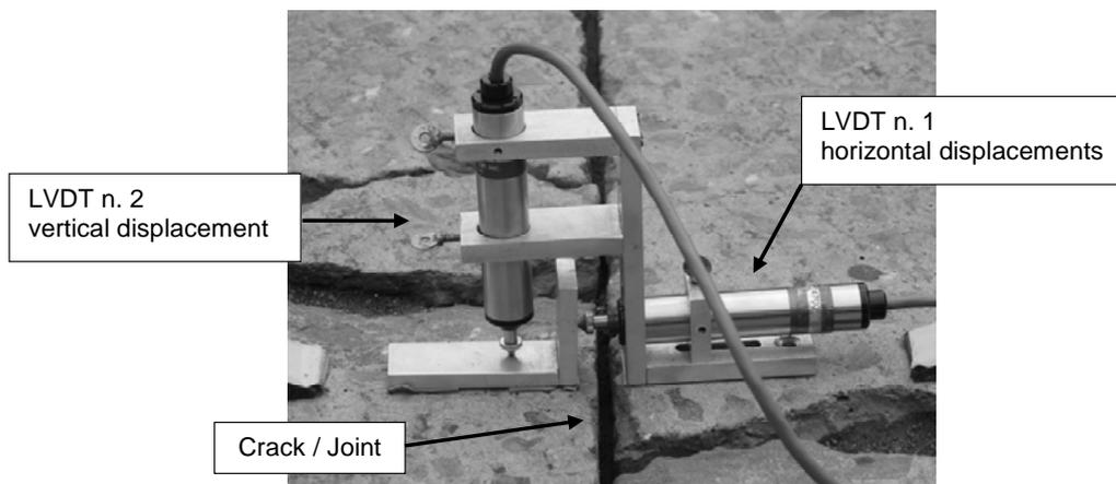
Figure 2: Crack activity meter
