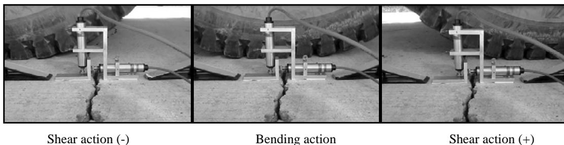
Figure 3: Wheel load stresses in a crack
