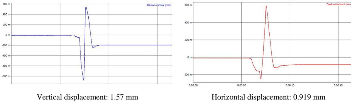
Figure 5: Vertical and horizontal displacement – station 163
