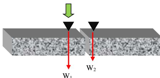
Figure 6: Load and sensors position for approach 1
